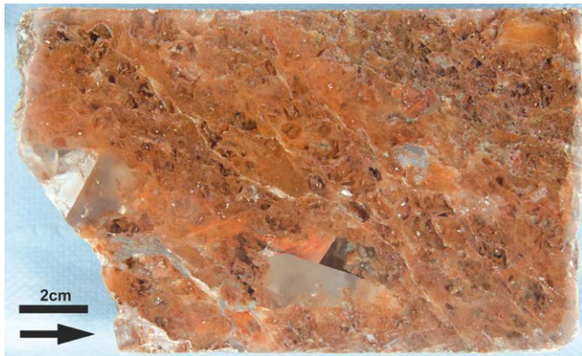
Fig. 10. Lower Tonbrockensalz (z4TSU): Polished surface of a core of the Go1004 (depth: 1808.30–1808.47 m); arrow points in drilling direction.
