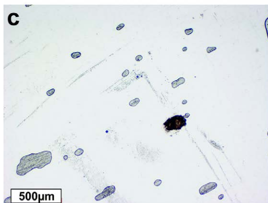
Fig. 12. Microphotographs of lower Tonbrockensalz (z4TSU): a) halite crystals with fluids on grain boundaries, b) elongated halite crystals, c) fluid trails within a halite crystal, d) zoom into (c) angular shaped fluid inclusions, all microphotographs with parallel polarizers.
