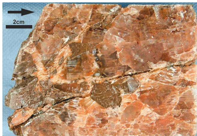
Fig. 11. Upper Tonbrockensalz (z4TSU): Coarse-grained rock salt with fractures, fibrous halite, and clay clasts; Polished surface of a core of the Go1004 (depth: 1814.30–1814.44 m); arrow points in drilling direction.
