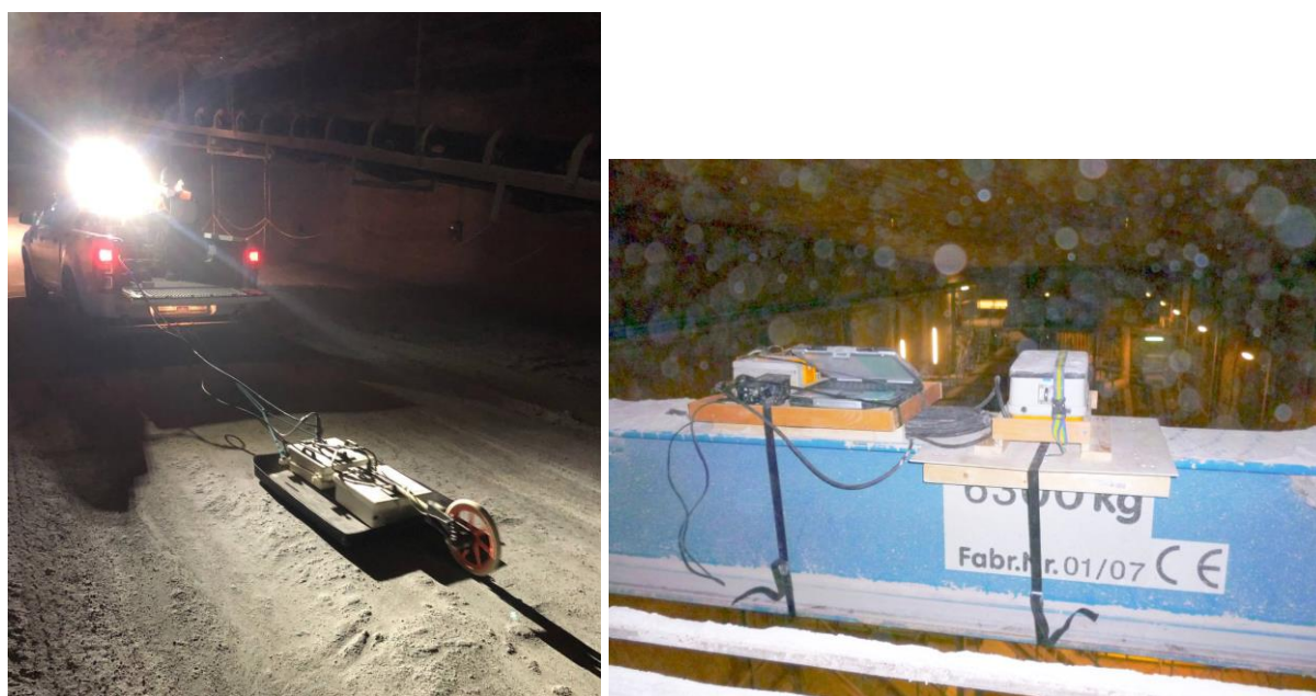
Fig. 1. GPR antennas pulled behind vehicle during floor-based survey (left) and attached to a gantry crane for roof-based survey (right).
